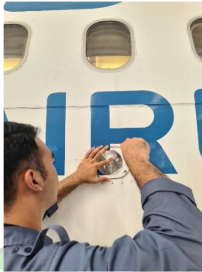
Gambar 4. 5 Replacement of the Lamp of the Wing and Engine Scan Light
