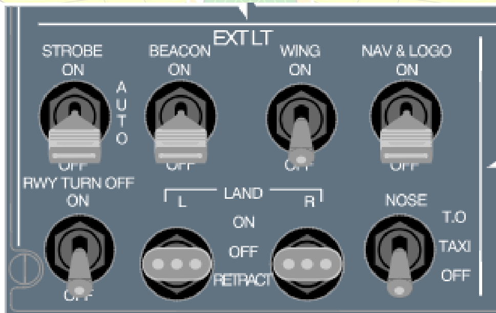
Gambar 3. 8 Overhead Panel Exterior Light
