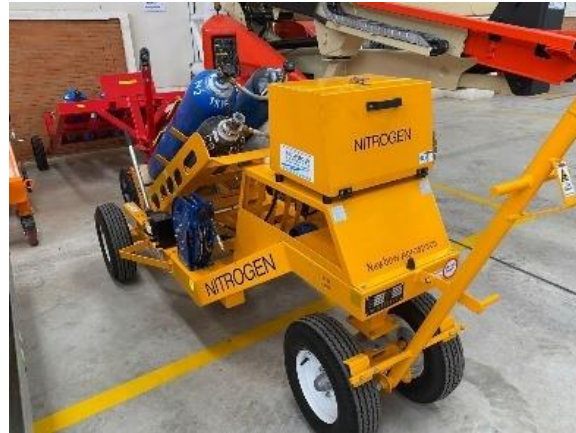
Gambar 2. 13 Nitrogen Service Cart
