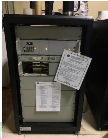
Gambar 3. 6 Transmitter ATIS Merk JOTRON
