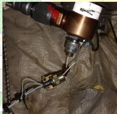
Gambar 4. 9 Broken Cable Connector B
