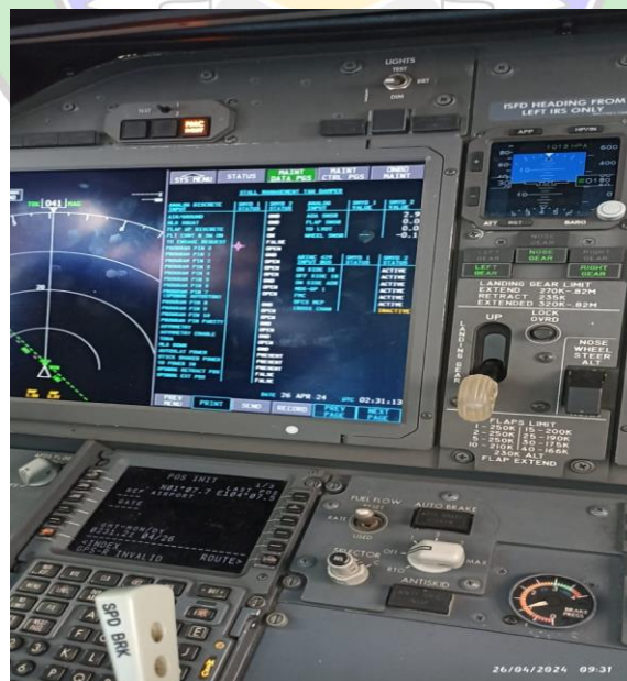
Gambar 4. 1 Fault Stall Management Yaw Damper
