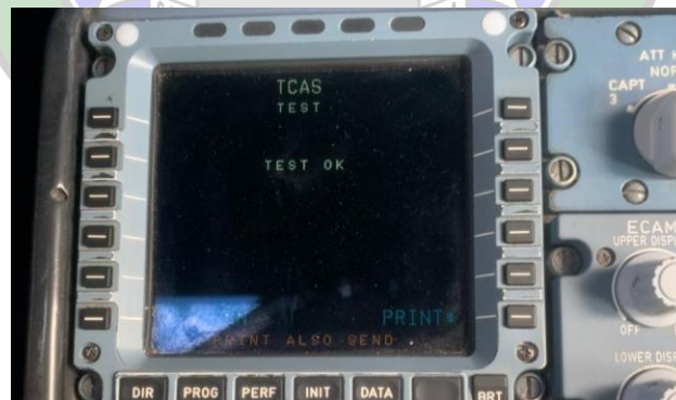
Gambar 4. 9 Functional Test TCAS
