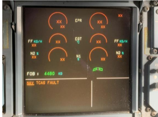
Gambar 4. 7 Fault Message Appear on Upper ECAM
