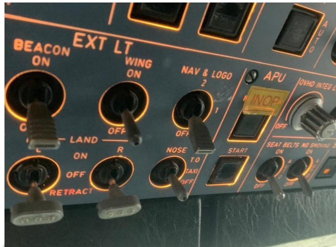
Gambar 4. 2 Operational Test Taxi Light
