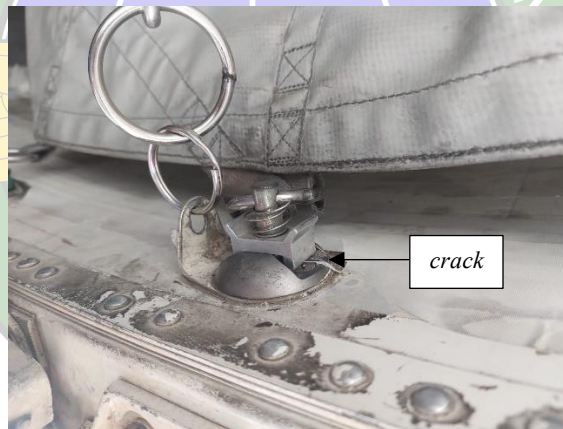
Gambar 4.1 Bracket Aft Cargo Lanyard Crack Sumber : Dok. Pribadi
