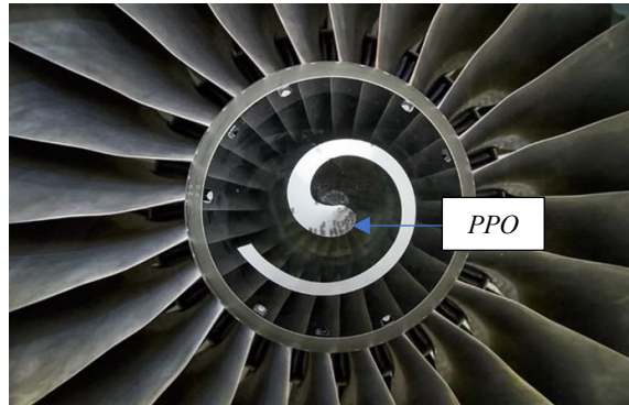
Gambar 4.3 Spinner Engine Paint Peel Off Sumber : Dok. Pribadi
