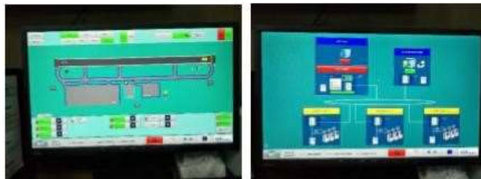
Gambar 4. 1 Display Airfield Lighting Control Management Systems Sumber : Arsip PT. Angkasa Pura I (Persero)
