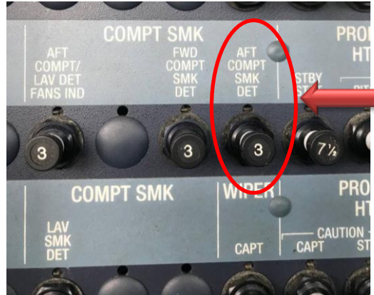
Gambar 4. 15 Circuit Breaker Smoke Detector
