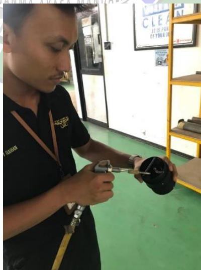
Gambar 4. 17 Proses Cleaning Smoke Detector
