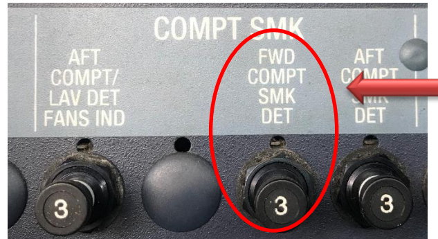
Gambar 4. 18 Circuit Breaker Fwd Smoke Detector
