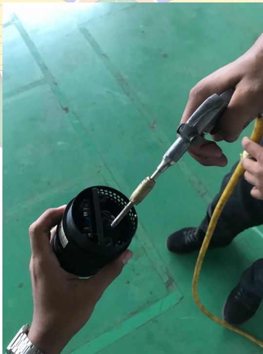
Gambar 4. 20 Proses cleaning Fwd Smoke Detector
