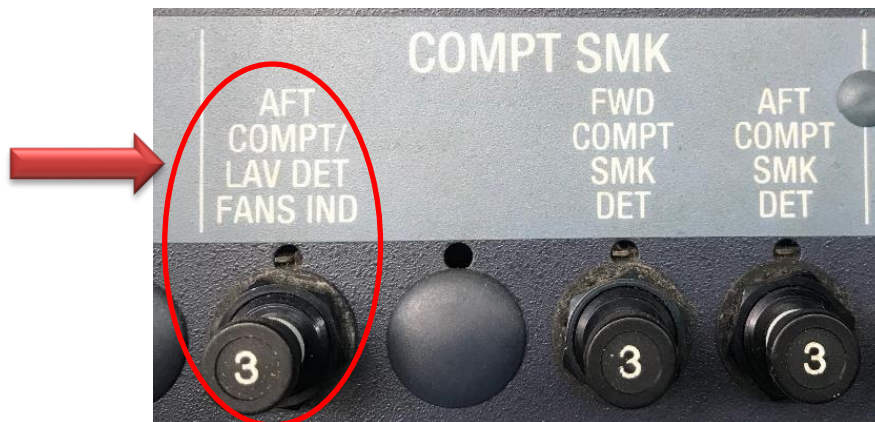
Gambar 4. 21 Circuit Breaker Lavatory Smoke Detector
