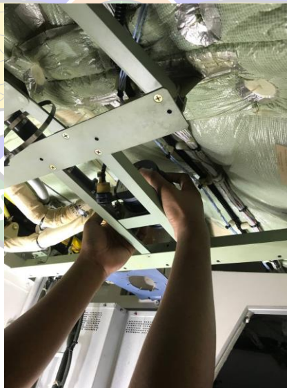
Gambar 4. 22 Remove Lavatory Smoke Detector
