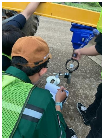
Gambar 4. 24 Proses Uji CBR Lapis Base Course
