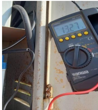
Gambar 4. 7 Hasil Pengecekan Panel Surya
