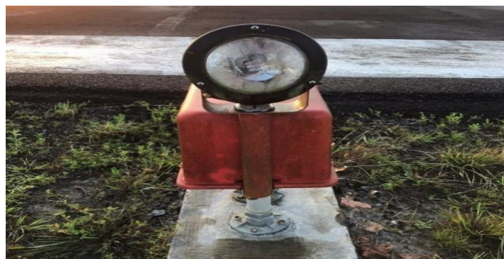
Gambar 2. 18 Runway Threshold Identification Light
