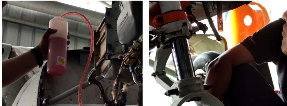
Gambar 4. 9 Proses shock strut servicing setelah proses re-assembly selesai
