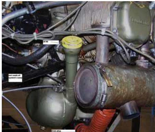
Gambar 3. 8 Basic wet sump oil system (sumber : FAA, Aviation Maintenance Technician Handbook, Powerplant Volum 2)
