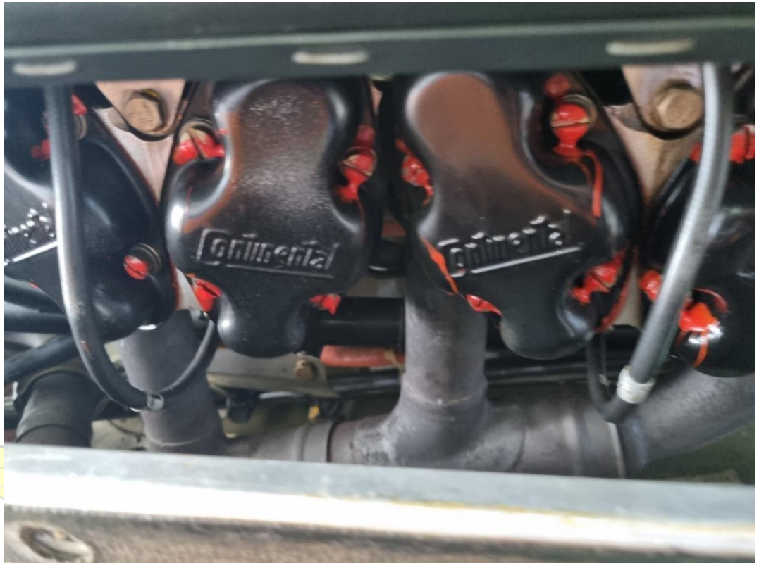
Gambar 4. 5 : Installation rocker box
