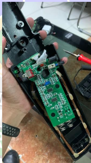
Gambar 3.18 Modul Hand Held Metal Detector
