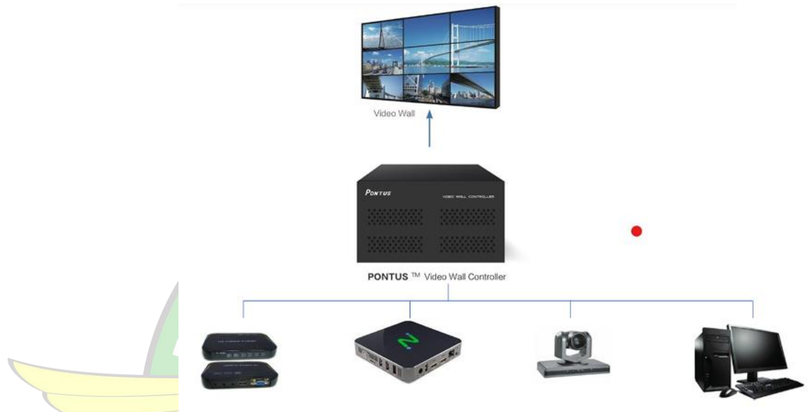
Gambar 3. 20 Topologi system video wall
