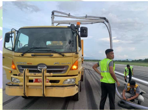
Gambar 4.11 Alat rubber deposit removal Water Blasting SK3000
