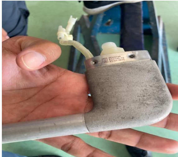
Gambar 4.12 Inspection Pitot Tube
