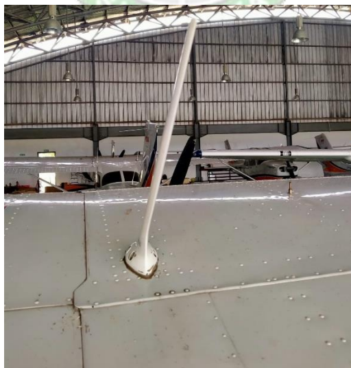
Gambar 4.7 Reassembly GPS Antenna
