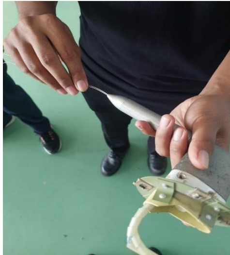
Gambar 4. 15 Inspection Pitot Tube
