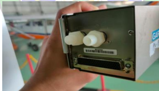
Gambar 4. 4 Diassembly GDC 74A
