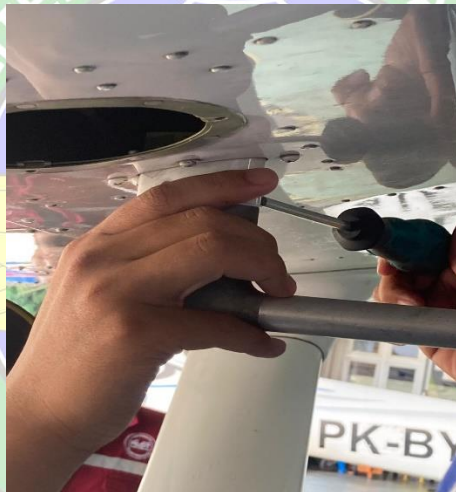
Gambar 4. 3 Visual Check Pitot Tube
