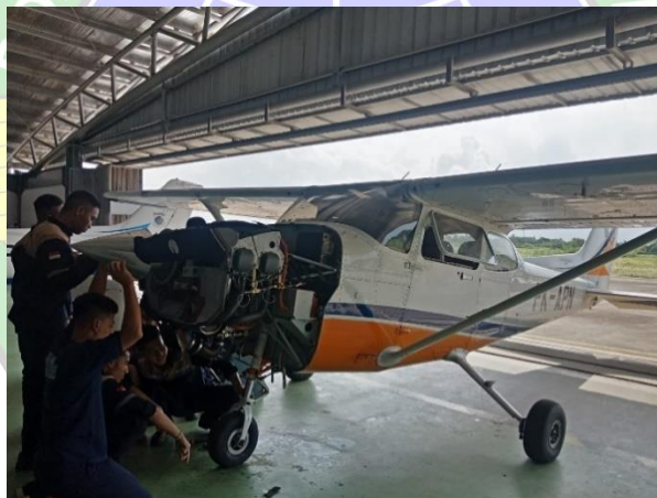
Gambar 3. 2 Maintenance Cessna 172S
