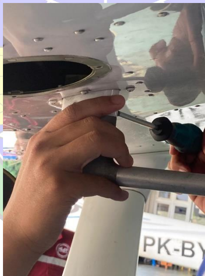
Gambar 4. 14 Disassembly Pitot Tube
