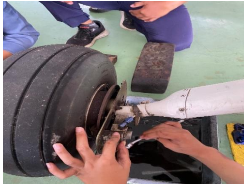
Gambar 4. 20 Install Brake Lining
