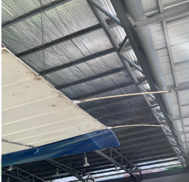
Gambar 3. 12 Static Discharge Cessna 172-S
