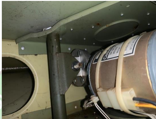
Gambar 4. 21 Replace Flap Motor
