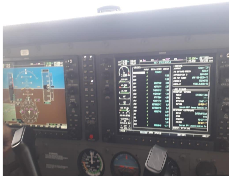
Gambar 4.16 System Status Page GDC normal
