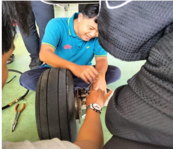
Gambar 4.20 Instal Brake Lining
