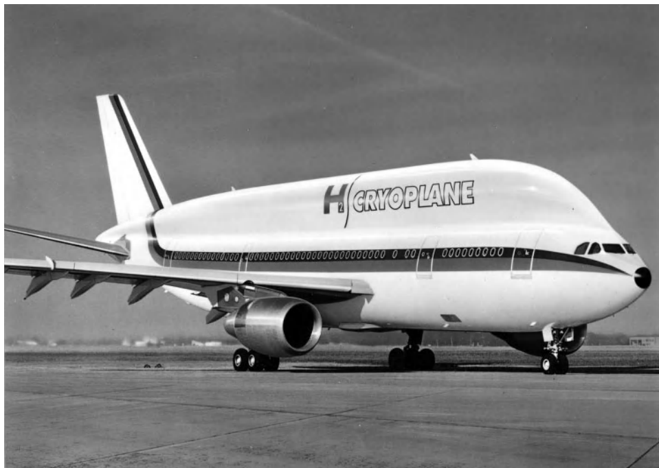
Figure 6.21 DASA Cryoplane wide body airliner with LH 2 propulsion. Reproduced with permission from Daimler-Benz Aerospace Airbus GmbH
