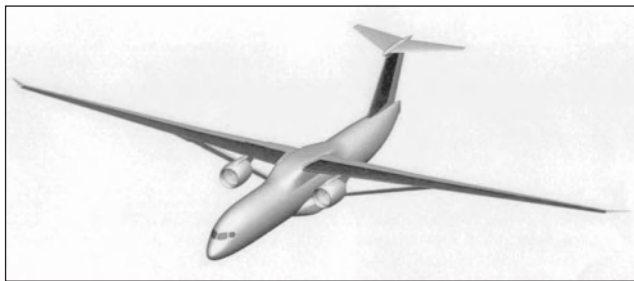
Figure 10.3 High span strut-braced folding wing concept described in NASA/CR-2011-216847
